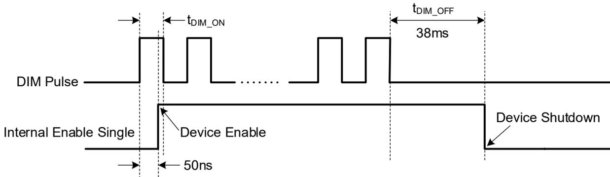
Figure 1. AS2472 DIM Time Sequence
