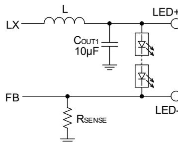
Figure 3. FB and LED+ Connect Circuit
