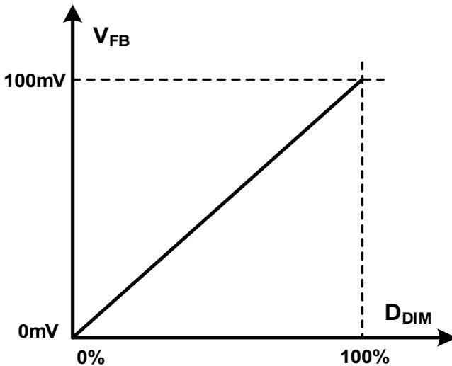
Figure 2. AS2472 Dimming Curve
