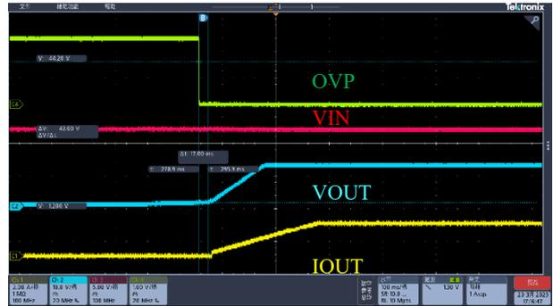
Input over voltage protection release
