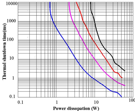
The power dissipation, with and without load, for selected start up time should not exceed the shutdown limits as shown in above figure.
