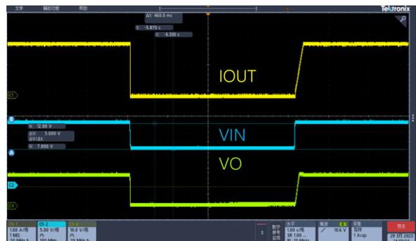
Input undervoltage protection and release
