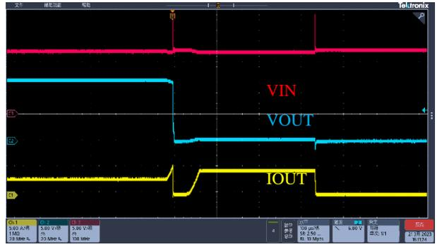
Output short circuit protection in normal operation
