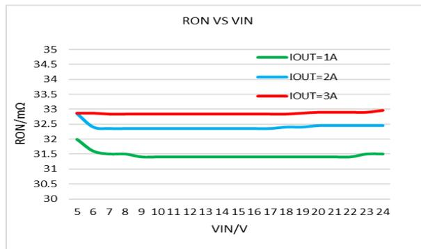
Internal on resistance vs VIN
